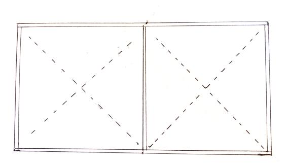
Floor is frame using 1" X 2" Furring strips and has a center divider. Cover floor with 1/2" Hardware cloth stapling to framework. Flooring is screwed in place 3" above bottom framework. The clean out trays sit on top of bottom framework.
