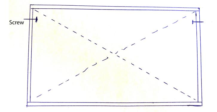
Doors are framed with 1" X 2" and covered with 1/4" Hardware cloth. Drill holes on opposite sides approximately 2" from outer edge. Fasten to frame using 2" Deck screws. Leave a little loose so door can pivot.
